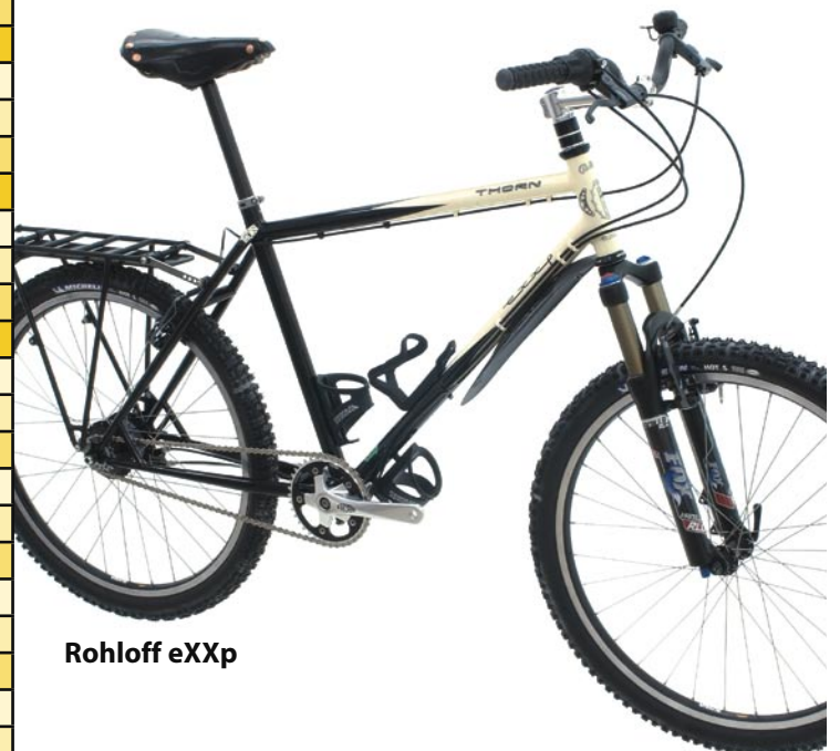
Rohloff eXp EX gear mech version
