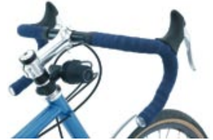
Rohloff twist grip mounted on Thorn's accessory bar, leaving room for a barbag, lights or computer
