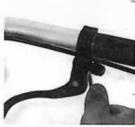
Open the hinged clamp of the top mount lever by-unscrewing the clamping bolt-with a 4mm Allen key.
