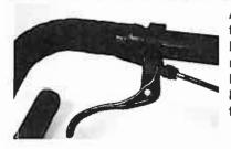
Attach the housing & cable to the brake, and set up the brake according to the manufacturers instructions. Re-wind the grip tape onto the handlebar and secure with tape.
