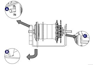
4. Locate the lock-washer (4), fulcrum lever (5) and guide nut (6), **Do not tighten nuts at this point**. Align the wheel, tension the chain and ensure the fulcrum lever (5) is leveled with the bracket.
