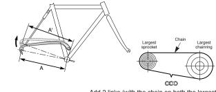
Add 2 links (with the chain on both the largest sprocket and the largest chainring)
