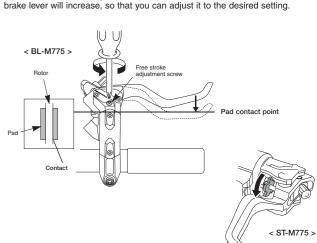
When the free stroke adjustment screw is loosened, the free stroke of the
