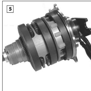
Lie the gearbox on its side and remove and dispose of the excess oil that is sitting in the hub casing.
