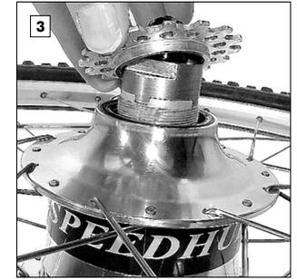
The sprocket can be removed over the sprocket tool. When only reversing the sprocket, clean the sprocket turn it over 180° and screw it back onto the cleaned and regreased thread of the driver in a clockwise direction. Tighten up the sprocket using the chain whip. If the sprocket needs to be replaced, simply screw the new sprocket tightly onto the driver.
