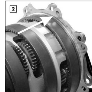
The new paper gasket (arrowed) must be fitted over the centering ridge of the hub cap. This is better accomplished when lightly greased. Align the holes in the paper gasket with those in the hub cap ready for the bolts later.
