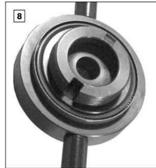
Place the new hub seal around the centering collar of the press tool.
