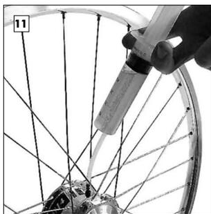
Refill the Rohloff SPEEDHUB 500/14 with 25ml of Rohloff SPEEDHUB OIL (see chapter "Service", paragraph 1. "Oil change") and refit a new drain screw (3mm allen key, tightening torque: 0.5Nm/4in.lbs.).
