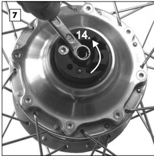
With an 8mm wrench turn the hexagonal peg in an anticlockwise direction until the end stop. Now the hub is in gear #14.
