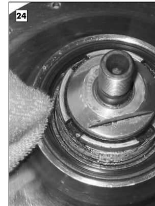
Remove the ring and the sprocket tool.
