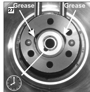
27 Make sure that the hexagonal peg sits correctly within the hole of the cable pulley (groove between the 7 and 8 o'clock positions). It may be necessary to alter the position of the cable pulley by a minimal amount. Place some grease between the cable pulley and the axle ring (arrowed). Replace the axle plate and secure into position with the six axle plate screws, tightening them in cross formation (Torx TX20, tightening torque: 3Nm/25in.lbs.).
