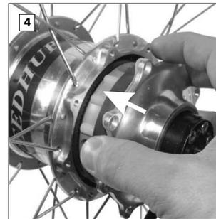
Hold the hub cap and the gearbox firmly and feed the gearbox into the hub casing until the hub cap touches the hub casing.
