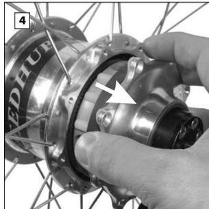
Draw the gearbox out of the hub casing. If this proves to be difficult, than gently tap the sprocket side of the gearbox with a rubber mallet to ease the process. CAREFUL! Excess oil could still leak out of the hub casing!
