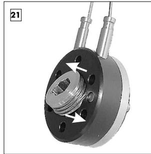
21 Pull the cable pulley up to the axle ring by pulling both ends of the hub cable equally. Push the cable pulley into a parallel position with the axle ring using the thumb (from outside) and index finger (from inside) whilst keeping the tension applied to both hub cable ends. The cable pulley then springs into the axle ring hole.
