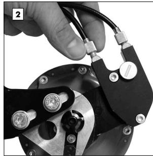
On the versions with an external gear mech the cable adjusters can be found on the cable box. This sits directly on the left hand side of the *Rohloff SPEEDHUB 500/14*. These cables are either routed along the seatstay or the chainstay of the frame.
