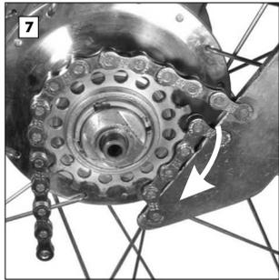
Refit the sprocket with the use of a chain whip.
