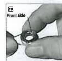
Grip the cable pulley with a free hand so that both ends of the hub cable are held in position. Hold this so that front side of the cable pulley faces up.
