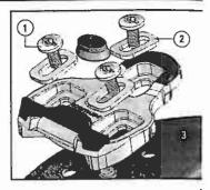
Step 5: once the cleat is suitably adjusted, check the tightening torque (within 5.5 - 6 Nm range)
